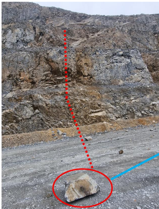
Rock fall at Top Moscow ramp that contacted LV0 989
