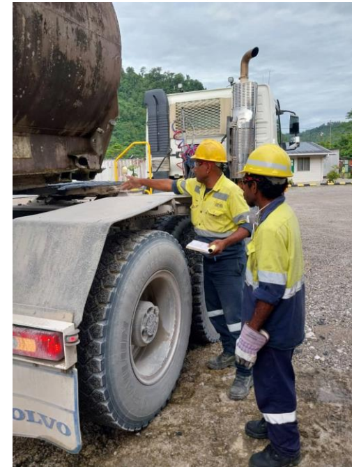
Operator, explaining / conducting Pre-start Checks and the Safe Operation of a Prime Mover when hooking / unhooking of Fuel or Waste Oil Tankers
