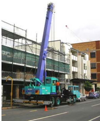
Figure 2 – Hazard striping on a mobile crane
