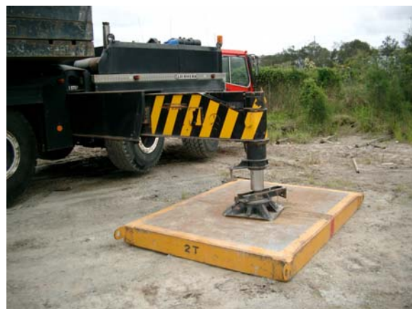
Figure 4 - Crane outrigger foot on bog mat
