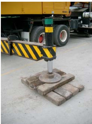
Figure 3 - Crane outrigger foot on timbers
