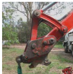
Figure 7 and Figure 8 - Lifting attachment with a closed eye on excavator
