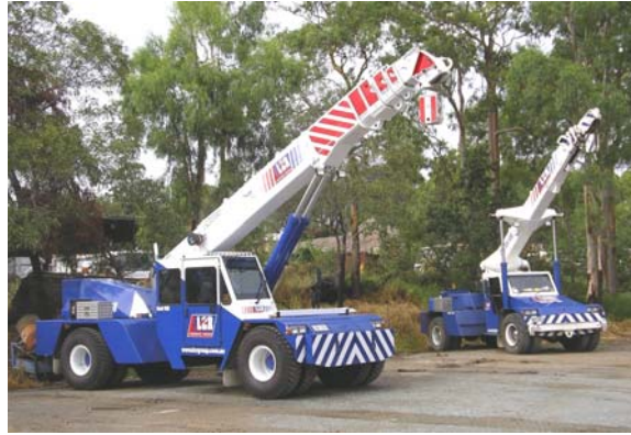
Figure 5 – Pick-and-carry mobile cranes (non-slewing hydraulic cranes)
