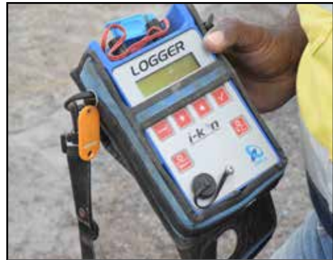
Typical Gas Monitor
