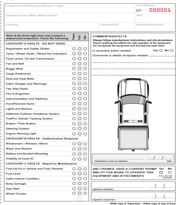
Vehicle operators shall conduct pre-start safety checks prior to first use of a vehicle each shift.
