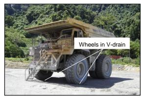
NOTE: All parked-up vehicles must be fundamentally stable before the operator leaves the vehicle.
